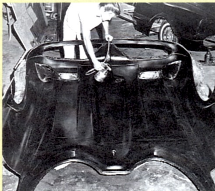
Barris used fiberglass molds to duplicate other Batmobiles off the original Ford Futura. Below: Spraying inside of the mold with black gel-coat.
